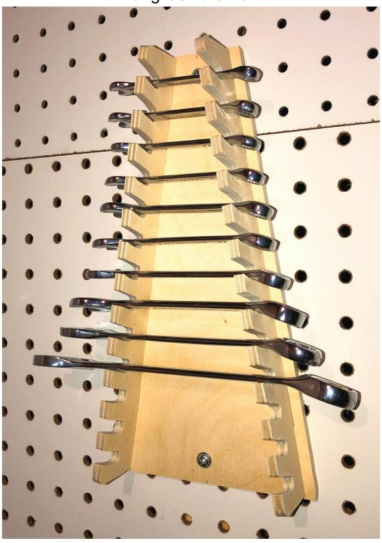
Note. If you plan to hang the wrench holder then you should install the brackets the opposite direction. In this case the slots are angled toward the small end.
