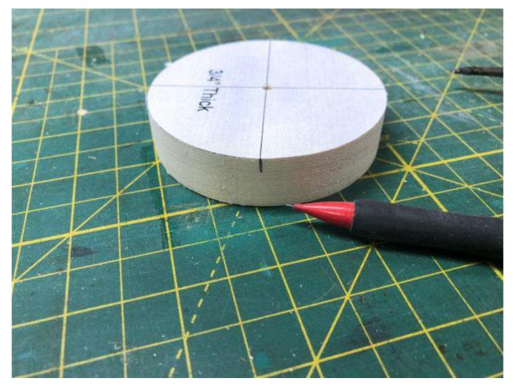
Use a straight edge to connect the lines just transfered from the pattern.
