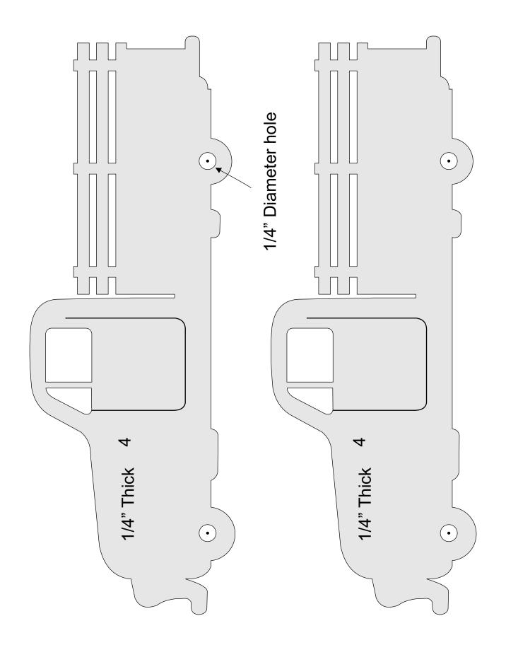
1/4" Diameter hole 2 1/4" Thick 1/4" Thick 1/2" Thick  $\odot$ 1/8" Thick ≈ 8 Use 1/4" wooden dowels cut to length for the axles. ന ന
