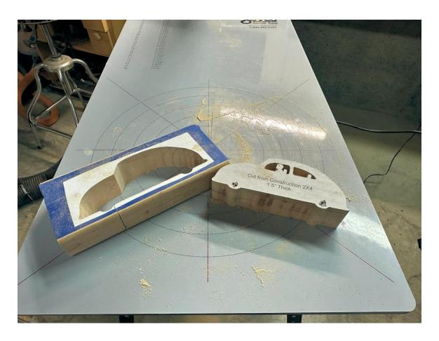
I used a #5 scroll reverse blade to cut the body and the fenders.
