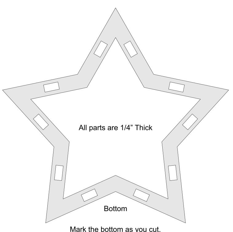
Mark the bottom as you cut. It makes it easier to assemble with the back board.
