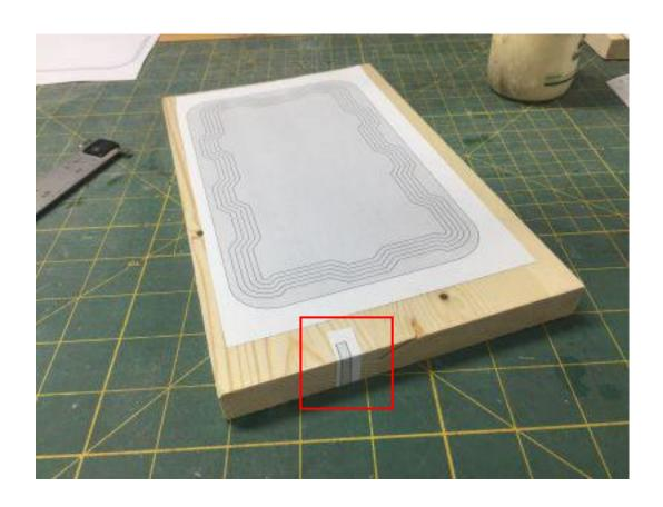
The pattern on the edge of the board is the angle guide. We will use it to set the silt of the table.
