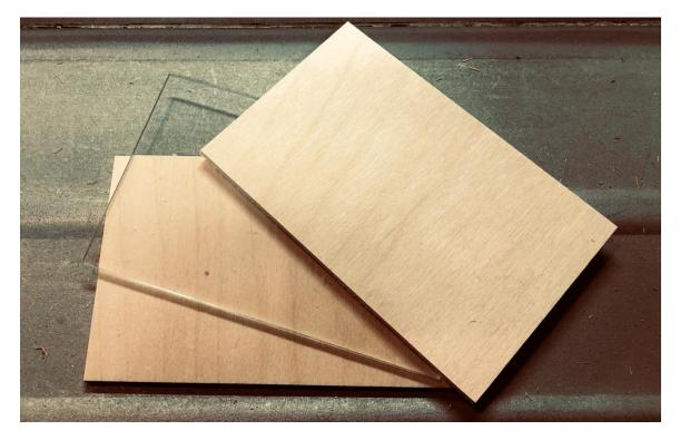
Sandwich the acrylic between two sheets of 1/8" plywood.
