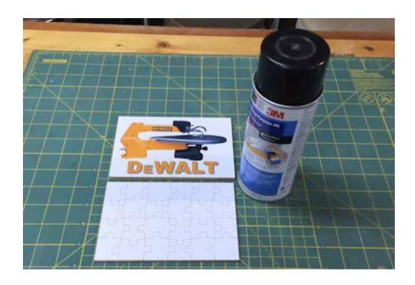
Stack the two pieces of plywood together with the pattern on the top.
