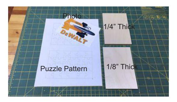
Use spray adhesive to apply the photo to the 1/4" thick Baltic birch plywood. Spray the back of the photo and the surface of the plywood for permanent adhesion.
