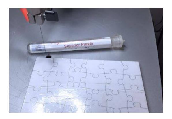
Begin cutting the pieces. After each piece remove the top piece of plywood with the pattern and discard.
