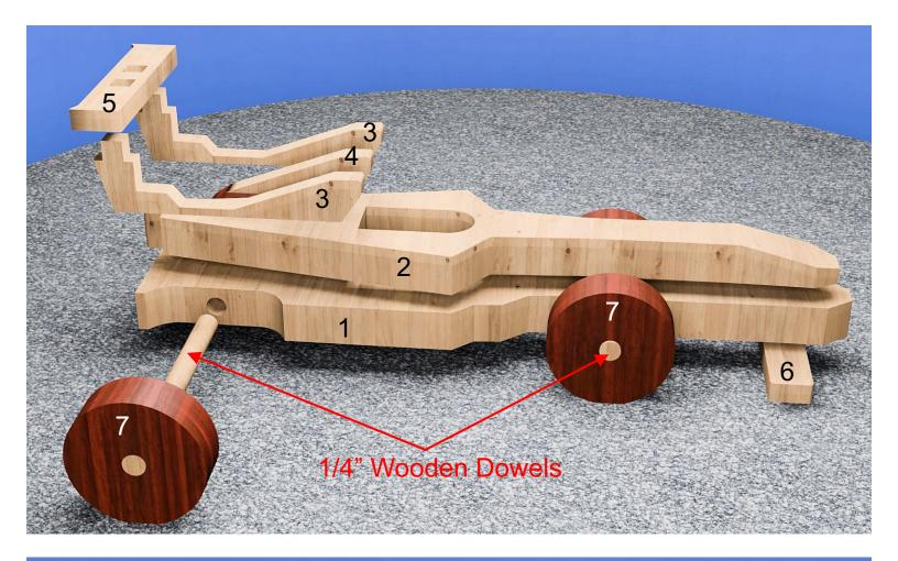
It is easier to drill the axle holes before you cut the lower body from blank.
