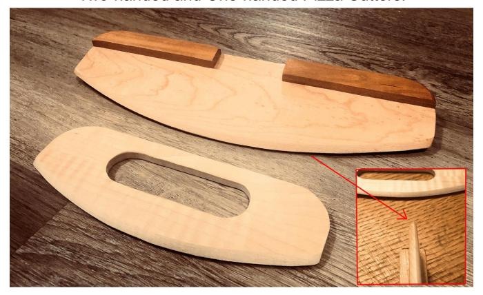
I used a disk sander to sharpen the cutting edge. You do not need to over sharpen the blade and make it fragile.
