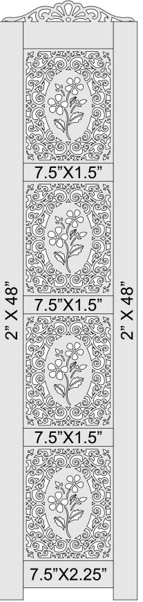
Use a table saw to cut groves for the panels to fit in the rails. The grooves need to be 1/4" deep and as wide as the wood you use for the panels.
