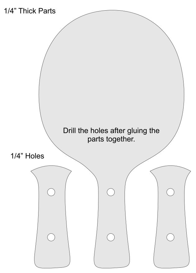
Plug with 1/4" diameter wooden dowels.
