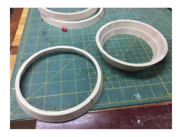
Carefully glue each ring together. Do not glue on the bottom until after we sand the bowl interior. It's easier to sand if the bottom is not attached.
