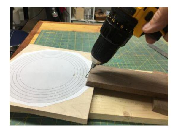
We need to drill the holes at the same angle that the table is tilted. Cut a board on the saw and use it as a guide to start the holes.
