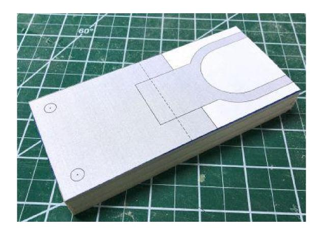
Drill a 1/4" hole at the way through the board. Do this before you cut at the scroll saw. A drill press works best.
