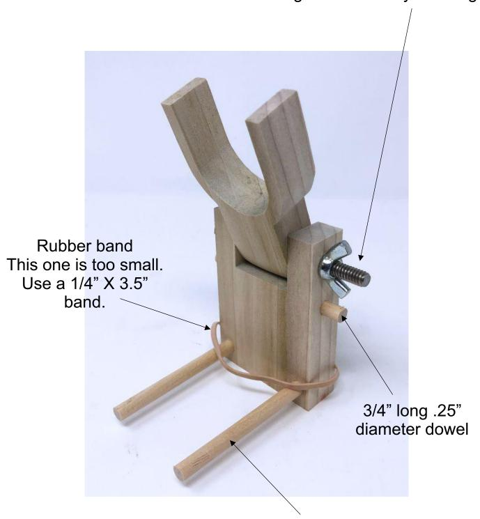
3" long X .25" diameter wooden dowels. Do not glue in place.
