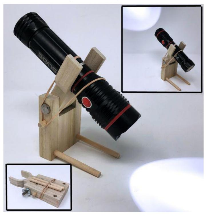
3" Bolt and wingnut Tighten until the yoke is tight.
