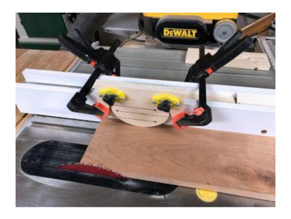
Above it is used as a hold down by clamping it to the table saw fence.
