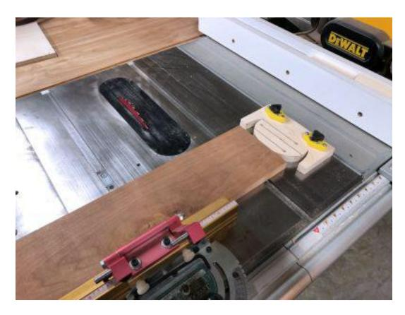
In this configuration it is used as a end stop for repeat cuts to the same length.
