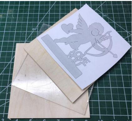
I use the sandwich technique to cut acrylic. I place the acrylic between two pieces of 1/8" or 1/4" Baltic birch plywood. I wrap the sandwich in blue painters tape. I then apply the pattern on the tape.
