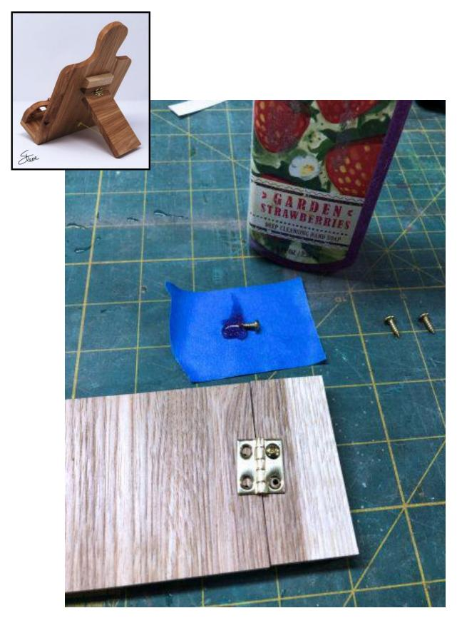
Tip: When driving small brass screws use a little soap on the threads. This will make it less likely to strip out the head of the screw. Make sure you use the correct size screwdriver.
