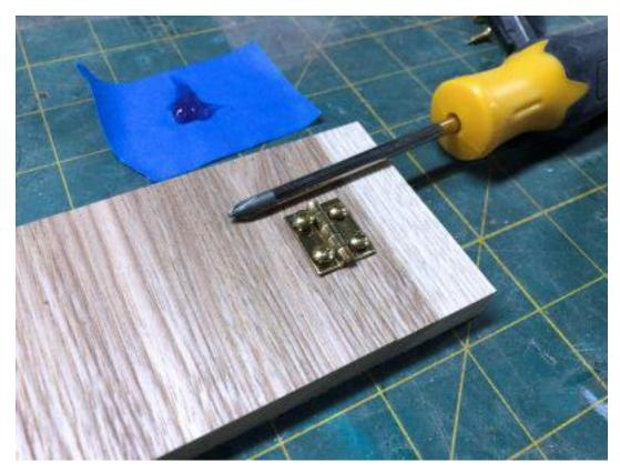
Start all the screws but do not tighten them until they are all started. This helps keep the hinge lined up. Pre-drill the holes with the correct size drill bit.
