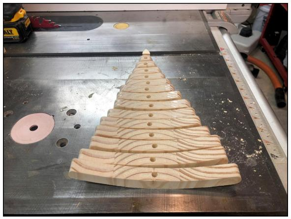
Mark and center drill for a 1/4" wood dowel.
