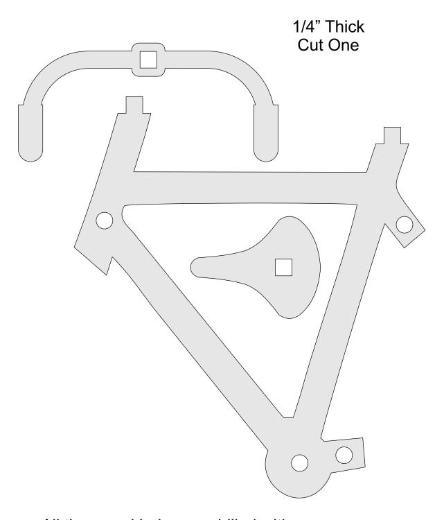
All the round holes are drilled with a 1/4" drill bit.
