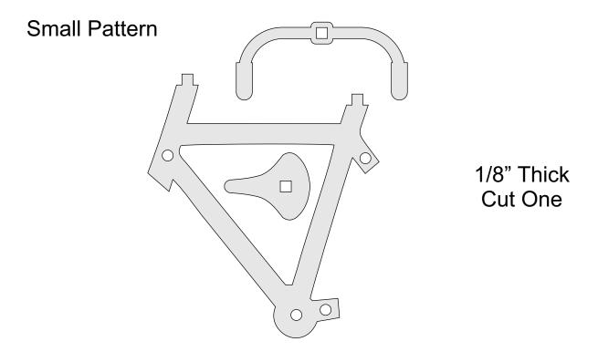
All the round holes are drilled with a 1/8" drill bit.
