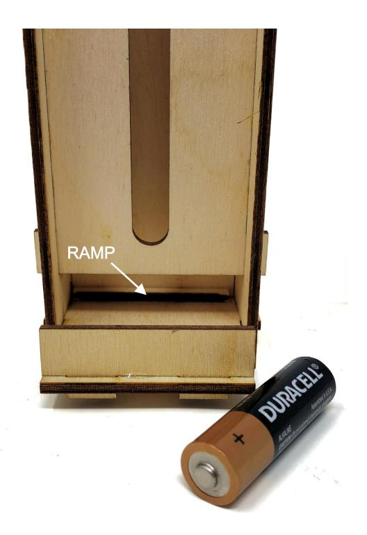
The ramp helps kick the bottom battery out on to the stop.
