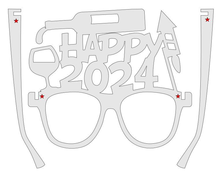
STACK CUT. Cutting 1/8" thick plywood on a scroll saw is difficult. It is best to stack cut two or more at a time to add a little resistance to the blade.
