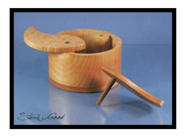
You can see in this picture how the dowel is used as the pivot for the lid pieces. Use 1/4" dowel. Drill the hole in the box just a bit larger so the dowel pivots freely.
