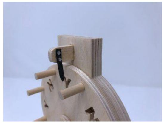
I cut off the end of a Tie Wrap(zip tie) for the paddle. I used two small brad nails to hold the paddle to the arm.
