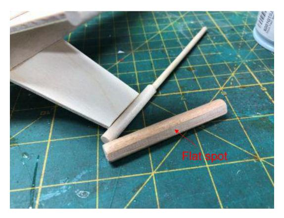
Cut the four 3/8" diameter engine dowels 2 3/4" long. Sand a flat spot on the side of the engine dowels.
