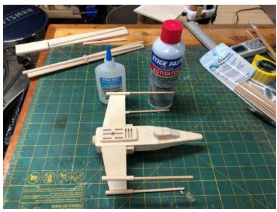
I used CA glue and activator to install the torpedo tubes on to the wings. Make sure they go on straight.
