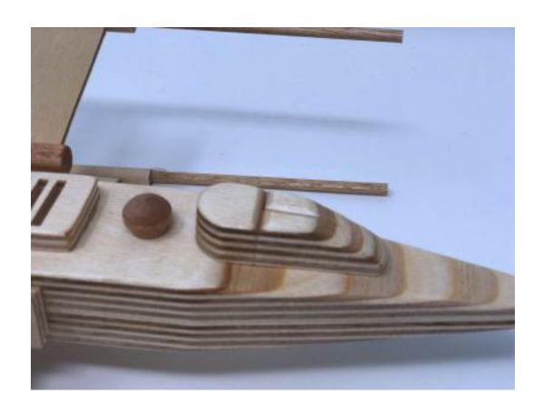
Cut the cockpit and contour. Note that I cut the cockpit into three parts and beveled the adjoining edges. Then taper the front of the cockpit to meet the body.
