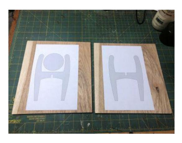
All the parts are cut from 1/4" thick wood.
