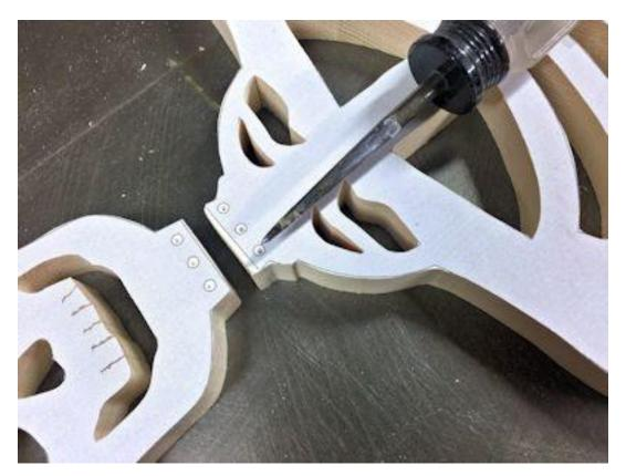
I marked the assembly holes with an awl and used a 1/8" drill bit to drill all the holes.
