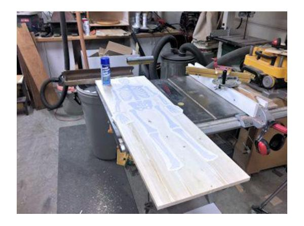
I used a laminated spruce panel purchased from Home Depot. It was 16" X 48". I laid out the patterns an made my cut marks to cut the board down to the correct size blanks.
