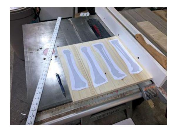
The pattern was then applied to each blank using spray adhesive.
