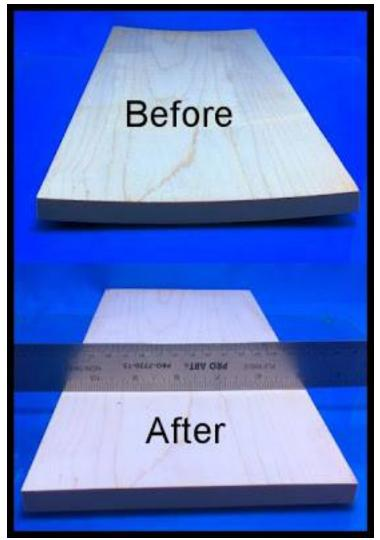
I am going to sticker this board for a couple of days and see if we can keep it from cupping again. I obviously added moisture content to the board and it needs to dry slowly on both sides.
