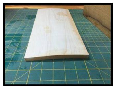
Now flip the board over on a flat surface so the edges curl down. Wet side down.
