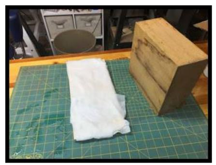
Apply the water soaked towels to the cupped side of the board. Edges curled up. Let the water soak in for a few minutes.
