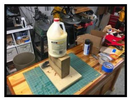
placed a piece of mdf to even out the weight on the board. Then a heavy block and gallon of glue. Hopefully as the wet fibers expand back the board will flatten out.
