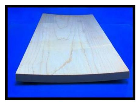
I could have possibly prevented this by stickering the boards like the picture below. This would have allowed the boards to dry evenly.
