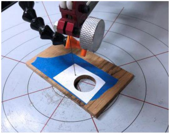
Not that the inside is close to a perfect fit it's time to cut the outside. Just freehand the outer circumference of the ring. This cut does not have to be anywhere near perfect. We are going to make it perfect at the sander. Shoot for no thinner than 2mm.
