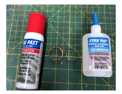
Use sand paper to rough up the surface of the steel insert. This allows the glue to bond better. Apply a thin layer of super glue to the interior of the wood ring. Spray the outside of the steel insert with activator.
