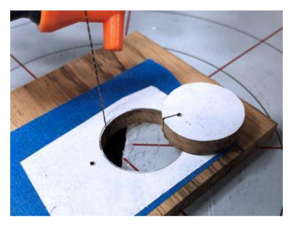
You have to cut carefully. You need to be accurate. If you have trouble throw it out and cut again. We are going to sand to fit but the hole cannot be too large at any spot.
