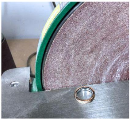
Now we have to true up the ring. Get it round. Go slow. This is also the time to make the wood the same thickness as the steel insert. It's easy to scratch the edge of the steel insert so be very careful.
