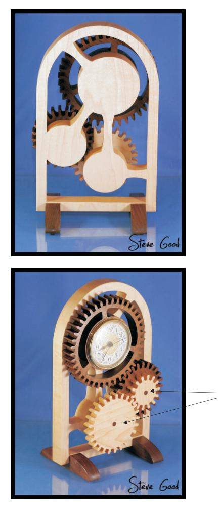
used 1/4" diameter wooden dowel to simulate the shaft. Just cut a small section and glue it in the holes of the two front gears.
