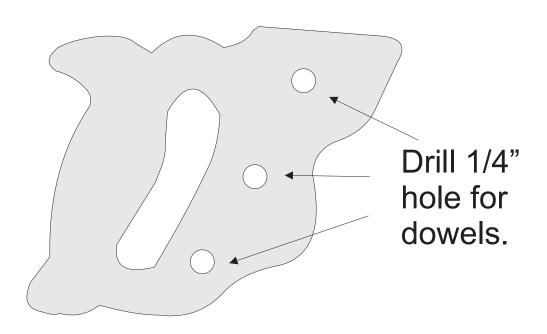
After you glue the handles to the saw, drill the holes for the rivets through the handles and saw blade. Hammer 1/4" dowel into the holes.
