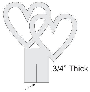
Drill for dowel before you cut the pattern. Use a 3/8" Drill bit.
