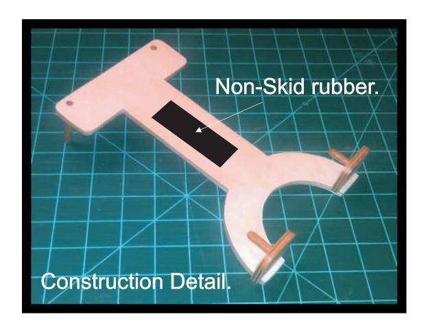
The cradle is designed not to be attached to the wheel. It sits on the two top dowels. This prevents driving with the cradle in place for safety.
