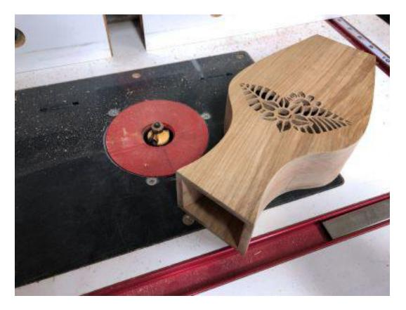
The edges need to be rounded over. Use a router table if you have one. Hand routing will work but be careful when you get near the top. As a last resort sand the round over.
