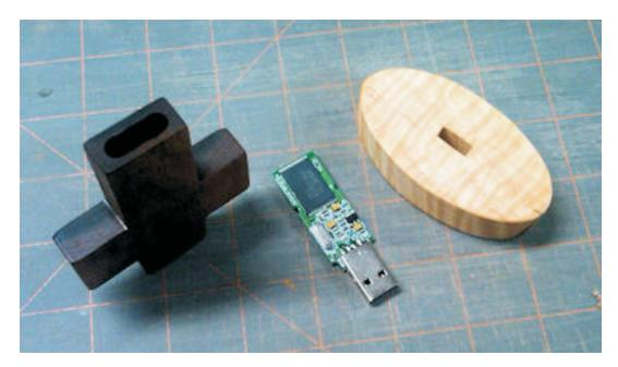
Test fit for a snug fit, Make sure the stick seats all the way to the end of the circuit board.
