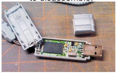
Carefully remove the circuit board from the case.
