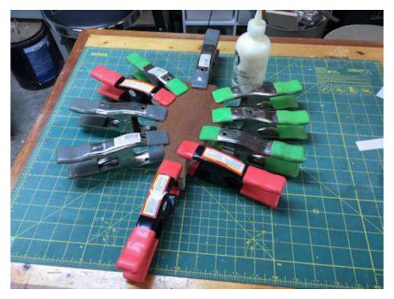
Clamp the parts. Notice I slightly over cut the front and back. This makes sanding the edges flush easier.
