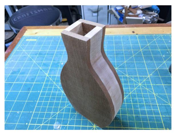
Sand the edges flush. Either sand or route a round over on the four sides. Do not round over the top or bottom. Finish as desired.
