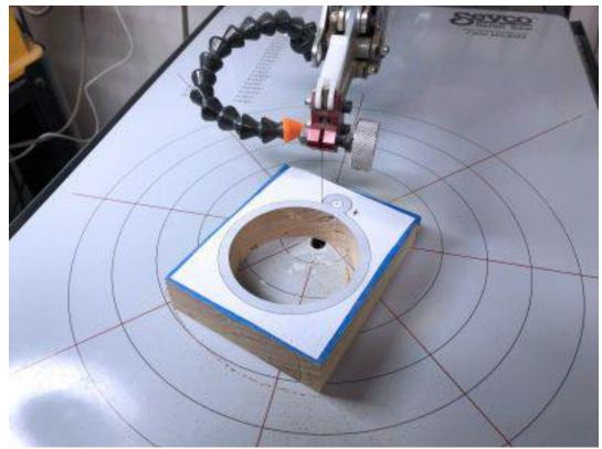
Carefully cut out each box. The more accurate you cut the less sanding you will have to do.
