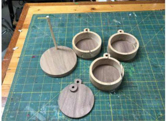
Cut a 1/4" diameter dowel to a length long enough to go into the base and through all three boxes plus the nut.
