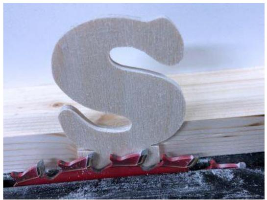
We will use the table saw to cut the tray slot. Set the height of the blade to match the height the tab on the bottom of the letters. Cut the slot then move the fense until the slot matches the thickness of the letters,
