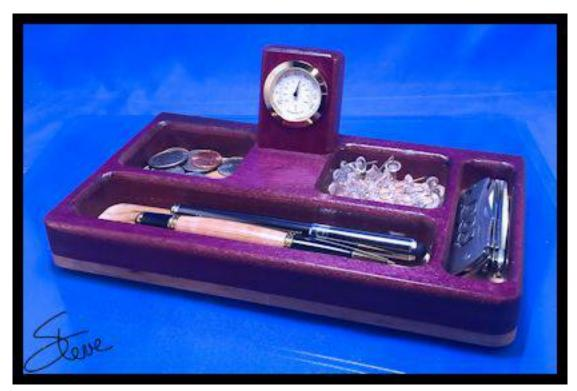
Requires a 1 7/16" mini clock insert. The mounting hole is 1 3/8" in diameter. You can cut the hole with the scroll saw or use a 1 3/8" forstner bit and drill the hole.
