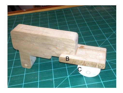
Glue parts C and B to body A both sides. Leave the pattern on part C to drill the axel hole through the body.
