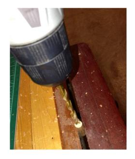
Drill 1/4" hole in both ends of 3/8" dowel.
