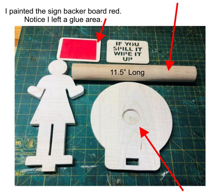
I used a 1 1/2" Fostner bit to drill the hole for the dowel. You could just as ealily drill a hole for a screw and attache the dowel with a screw from the bottom.
