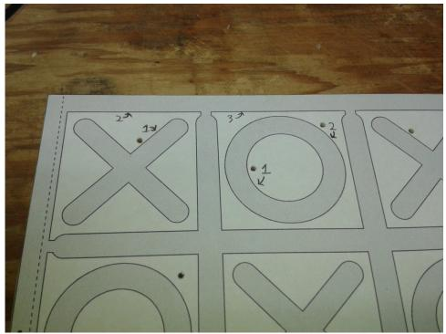
The above image shows the order to cut the pieces. Cutting in this order keeps you from having to cut from a small piece of wood, as it keeps it so you are always cutting from the whole 5 1/2" square.
