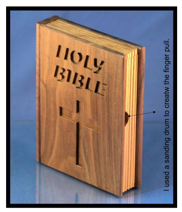
The front cover is two 1/8" thick boards glued together after the fretwork is cut to make a 1/4" thick front cover.
