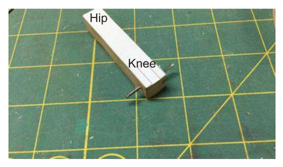
The joints will be pined by small nails. Drill the hole for the knee joint before you cut the slot.
