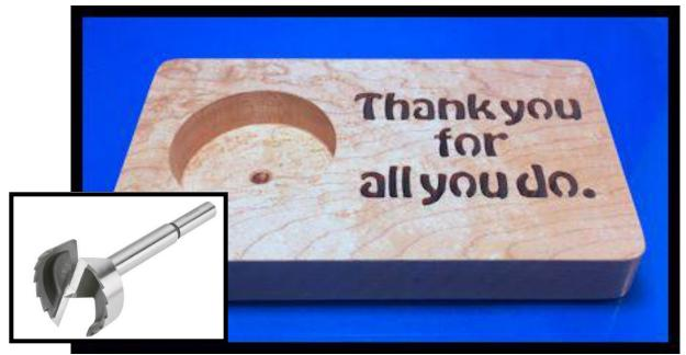
The clock insert mounting hole can be cut with your scroll saw. You may find it easier to use a 2 3/8 inch forstner bit like I did in the above picture. <u>Here is a link</u>.
