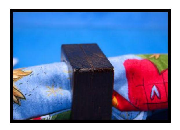
After you cut the pattern out turn the wood on it's edge and cut the slot for the card. Notice that it is at a slight angle.
