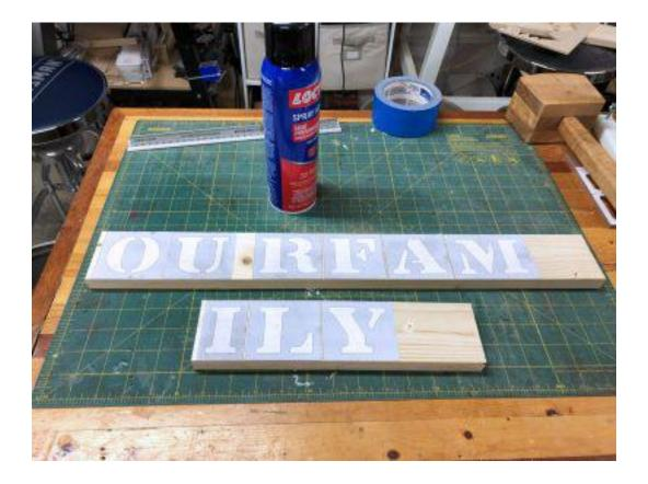
Use spray adhesive to attach the patterns to the board.
