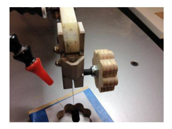
Remember to use this knob with caution. There is never a reason to over torque the clamp. It the blade is slipping you have another issue. Normal tightening should hold the blade in place.
