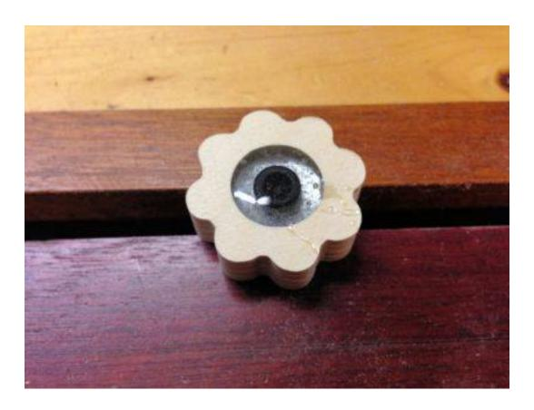
Fill the recess with the epoxy. Let it cure 24 hours before use. In the picture above I let the epoxy get into the head of the screw. You might want to cover the hear to keep it free of epoxy. That way you han use the allen to tighten the lock nut if necessary. In the install knob below you can see it was left open.
