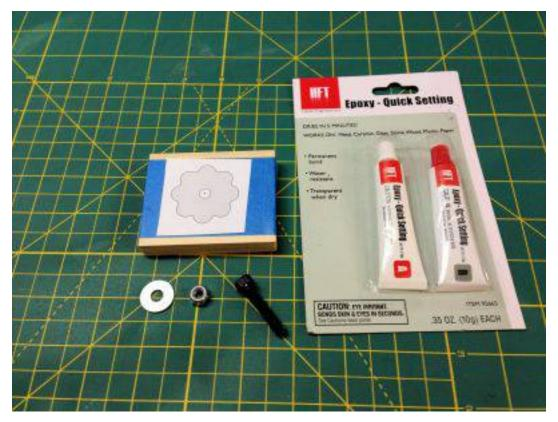
You will need: 1/2" thick Baltic Birch Ply M6-1.00 X 30 Socket Hd Cap Screw. Lowes #08326 71223 M6-1.00 Nylon Class 8 Lock Nut. Lowes #08236 71203 M6 x 18 Fender Washer Lowes #38902 00290 Two part epoxy This pattern.
