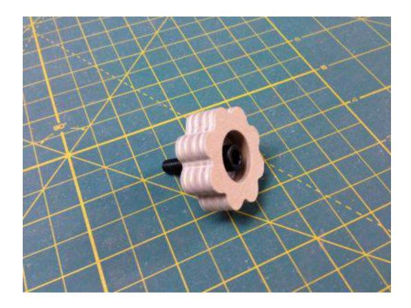
If you drilled just a little over half way the head of the screw will be below the knob surface. Mix up some two part epoxy and stir it for the required time.
