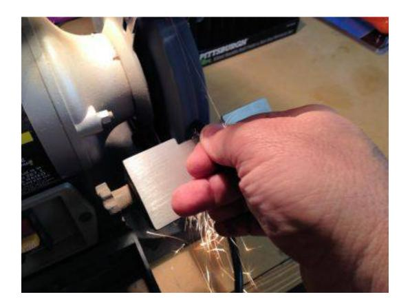
Use a grinder or a sander to flatten the tip of the screw. It is important to get it flat and square. It you have trouble with the blade slipping or being damaged then flatten it more.
