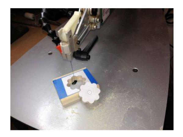
Apply the pattern to the Baltic Birch ply and cut the knob out.
