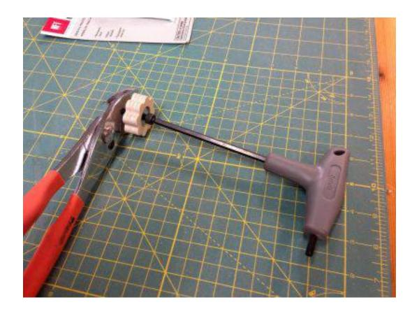
Tighten the screw assembly tight. It requires a 5mm allen for the 6mm screw.
