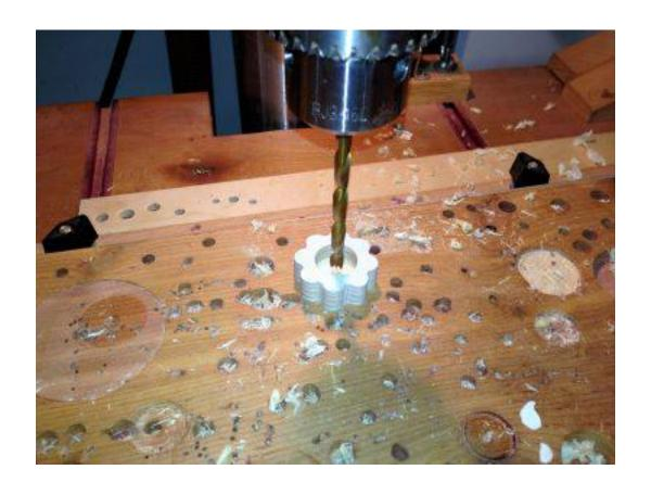
If you have standard drill bits a 1/4" bit will work fine. Drill the rest of the way through the knob.
