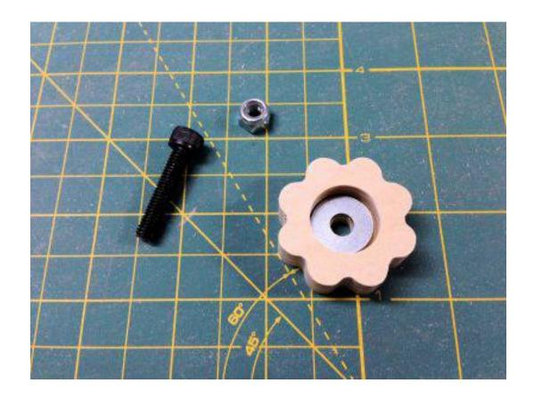
Install the washer and the screw into the cutout. Start the lock nut on the end of the screw.
