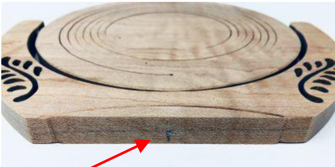
Brad nail used as a pivot on the foot.
