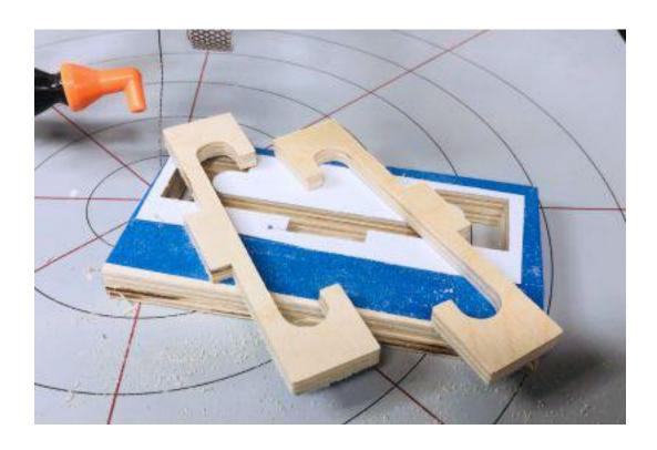
Spacer, item 5 has changes since the prototype was cut out. There is now a piece cut out of 5 to allow 6 more rotation.
