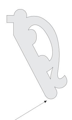
Sand this edge down to adjust the tilt of the easel. It needs to tilt back enough to support the weight of the displayed item.
